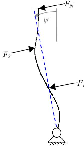
Figure 6. The model beam loaded and deformed. The reference line, shown dashed, coincides with the lowest beam reference position.  $\psi$  is the small angle through which the reference line is displaced.
