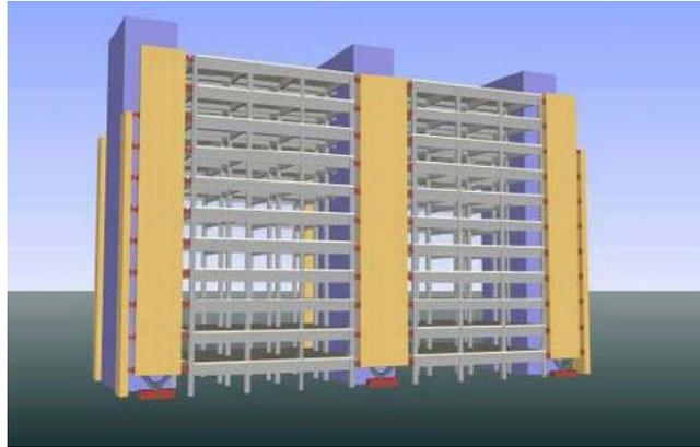
Figure 9. A model of the retrofitted case study building. Yellow represents new structure. (Wada *et al.* 2009)
