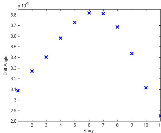
Figure 15. The story drift angles of the case study, with the maximum occurring at the 6<sup>th</sup> story.
