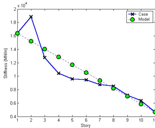
Figure 12. The case building story stiffnesses compared with the linear model
