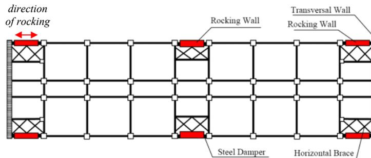
Figure 10. A plan view of the retrofitted case study building. Red rectangles represent rocking walls. (adapted from Wada *et al.* 2009)
