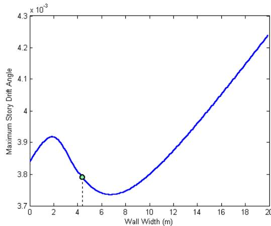
Figure 14. Maximum story drift angle of the modeled case study building, against rocking wall width (m), using 6 rocking walls. The location of the 4.39m-wide walls used in the case study is marked.
