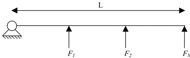
Figure 4. Model of the free rocking wall.
