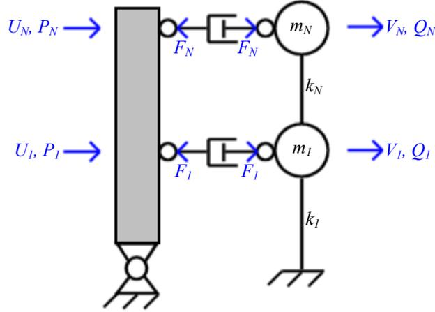
Figure 7. The rocking wall-building system model with forces and displacements required to complete the analysis
