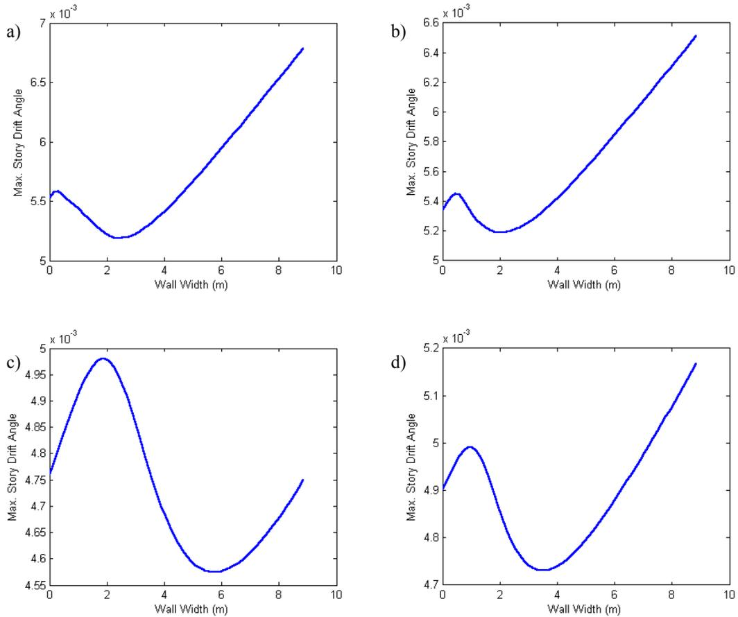
Figure 8. Functions of inter-story drift angle vs. wall width, where two identical rocking walls are used. The benchmark buildings represented have the characteristics a)  $N=6$ ,  $d=100\%$ ; b)  $N=7$ ,  $d=50\%$ ; c)  $N=9$ ,  $d=0\%$ ; d)  $N=10$ ,  $d=25\%$
