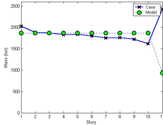
Figure 13. The case building story masses compared with the top-light constant model
