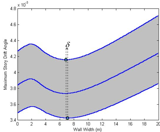
Figure 16. The rocking wall design function of the case study building compared to cases where all story stiffnesses are modified  $\pm 10\%$ . The central line is the case study, the upper with stiffnesses decreased by 10%, and the lower with stiffnesses increased by 10%. The change in the minimal width  $\delta$  is only 0.2m.
