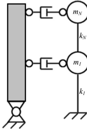
Figure 3. The statically condensed rocking wall-building system to be modeled.
