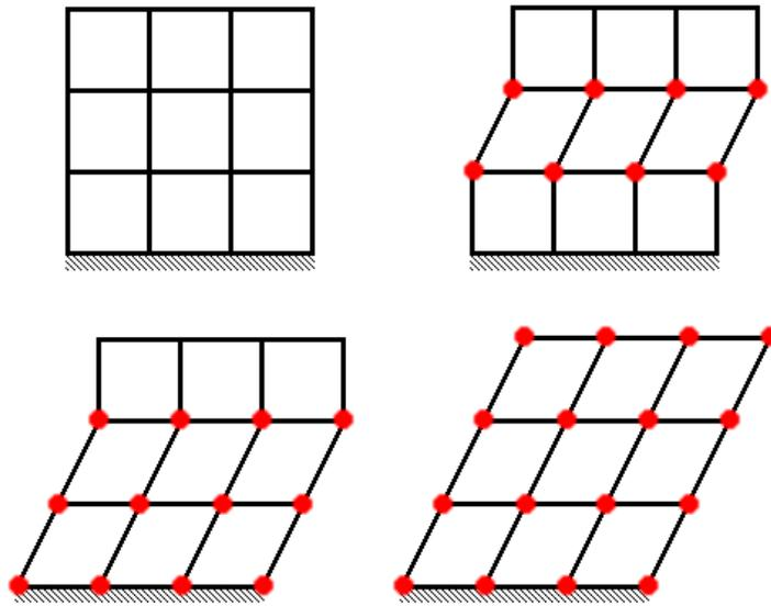
Figure 1. Schematic of a structural frame and its pushover failure modes. Red dots indicate plastic hinges.
